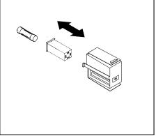
**3** Rotate line voltage selector and reinstall so correct voltage appears in fuse holder window.
