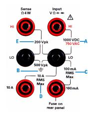
**Note:** The front-panel terminals and current protection fuse are shown above.
