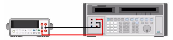
For range  $\geq 1 \text{ A}$ , Input  $\geq 3 \text{A}$
