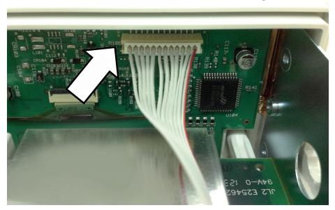
8 Disconnect the individual front panel wires as shown in the figure below:
