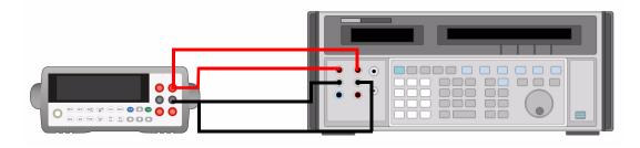
2-W resistance without compensation (For range 1 M $\Omega$  ~ 100 M $\Omega$  )
