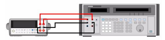
4-W resistance without compensation (For range 1 M $\Omega$  ~ 100 M $\Omega$  )
