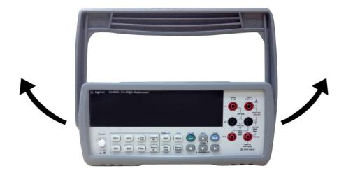
**3** Remove the instrument bumpers. Pull from a corner and stretch the bumpers off the instrument.
