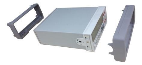
**4** Remove the rear bezel. Loosen the two captive screws in the rear bezel and remove the rear bezel.
