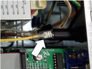
**10** There is now enough space to allow the side of the front panel to be pried from the chassis and removed as an assembly.
